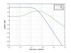
For disturbances at frequencies between 0.38 rad/s and 15 rad/s can appear saturation. Do not need to consider higher frequencies (no control there).
